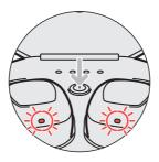
Note: While charging, the earbud indicator light should turn red. When the earbud is fully charged the indicator light will automatically turn off.
